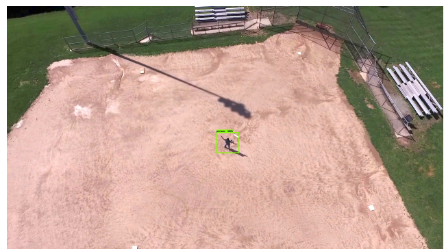
Fig. 2. Single frame of a human subject performing the “Move Right” gesture. This high-resolution video frame shows a human subject at a distance in a view from a UAV. We are actively exploring gesture recognition techniques for UAV control, and any such algorithm will likely need to localize the human subject before (or in conjunction with) classifying the gesture.
